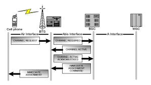
Figure 3. Channel assignment process in GSM
