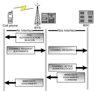
Figure 5. DOS-resistant channel assignment process in GSM
