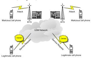
Figure 4. Denial of service attack in a GSM network
