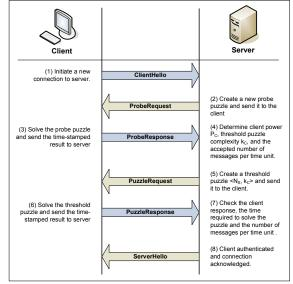
Fig. 4. Schematic of an authentication protocol protected by adaptive threshold puzzles
