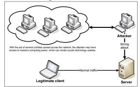
Fig. 3. Schematic of a strong attack on an authentication protocol protected by client puzzles
