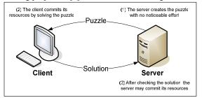
Fig. 1. Principle of the client puzzle protocol
